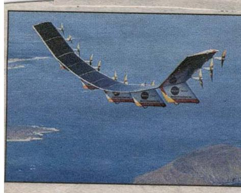
ing wing, which is 247-foot long, eight feet wide, and has 14 propellers, to a record 100,000 feet later this summer. The experimental aircraft, piloted via computer, is being developed by NASA and AeroVironment Inc.
